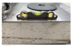
Using a level, ensure the scale tank is level both side to side and front to back. If the tank is not level, this could result in an unstable or inaccurate reading.
